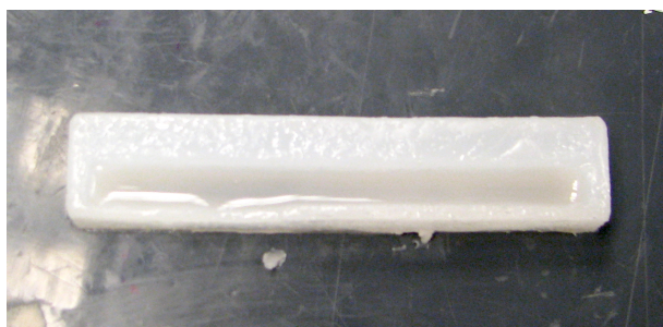
(a) Silicone Mold. Liquid wax is poured into the well and a silicone top is sealed on.
