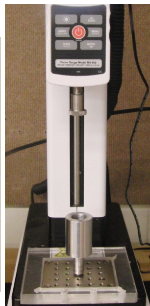
(b) The Mark-10 Gauge with aluminum mount.
