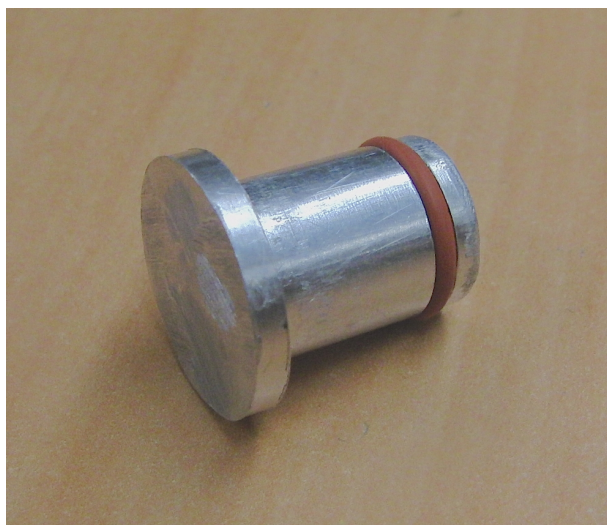
(a) The aluminum cap. O-ring fits very well in groove.
