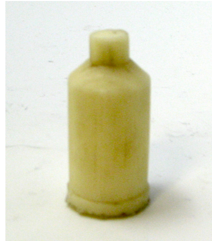
(b) Assembled Actuator. Piston moves freely up and down.
